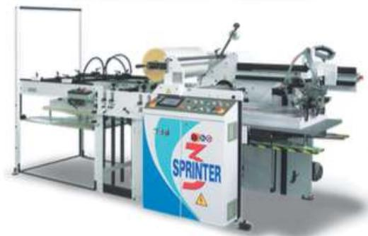
Thermal laminating machine (DRY), ideal for offset printer with integrated finishing.
